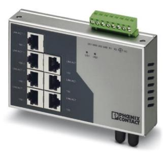
Ethernet Switch, 7 TP RJ45 ports, 1 FO port, 100 mbps full duplex in ST-D format, automatic detection of data transmission rate of 10 or 100 mbps (RJ45), autocrossing function
